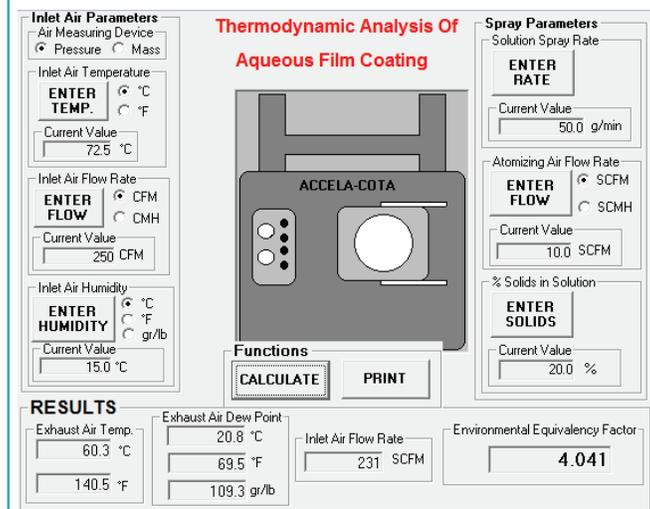
The EEF is a relative measure of the rate at which water evaporates from the surface of the tablet bed (higher values indicate drier conditions), and is determined based on convective heat and mass transfer calculations.<sup>2</sup> Maintaining a similar EEF value enables equivalent drying conditions to be achieved across multiple pans and coating scales. Tables 1 and 2 indicate the process parameters and the EEF values used for the coating trials at pilot and production scale respectively.
