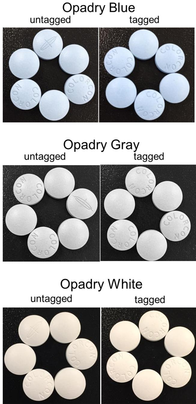
**Figure 3. Comparison of Gloss for Tablets Coated with Tagged and Untagged Opadry**
