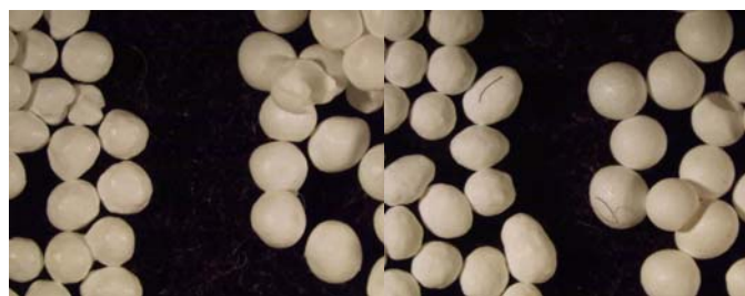
Figure 3: Optical Microscope Images of Pellets Before (MPs on the Left) and After Exposure to pH 1.2 (MPs on the Right): (A) without Fumed Silica; (B) with 1.0% Fumed Silica Sprayed
