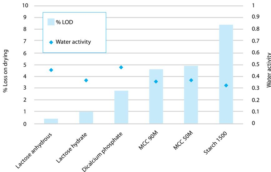
**Figure 5:** Moisture content and water activity of common tableting excipients. Moisture content encompasses all water present, while water activity discerns free and bound water. Only free water is available for reaction, while bound water is not readily available for chemical reactions (7)
