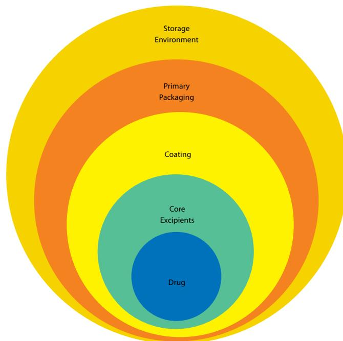
**Figure 1:** Levels of formulation development and product design that impact moisture protection
