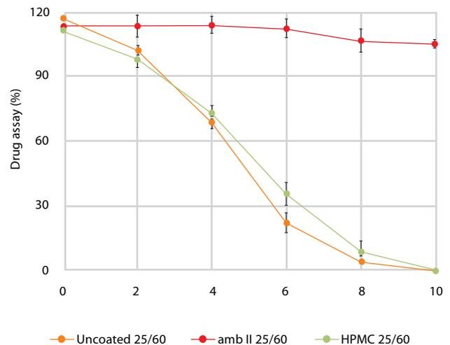
**Figure 4:** In-use stability of clavulanic acid. Tablets placed in a pill sorter and stored at 25°C/60% RH for 10 days. Tablets coated with Opadry amb II remained stable for the duration of the drug regimen
