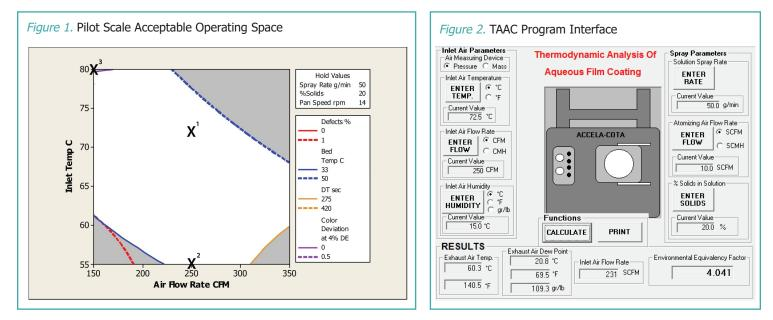
The EEF is a relative measure of the rate at which water evaporates from the surface of the tablet bed (higher values indicate drier conditions), and is determined based on convective heat and mass transfer calculations.<sup>2</sup> Maintaining a similar EEF value enables equivalent drying conditions to be achieved across multiple pans and coating scales. Tables 1 and 2 indicate the process parameters and the EEF values used for the coating trials at pilot and production scale respectively.
