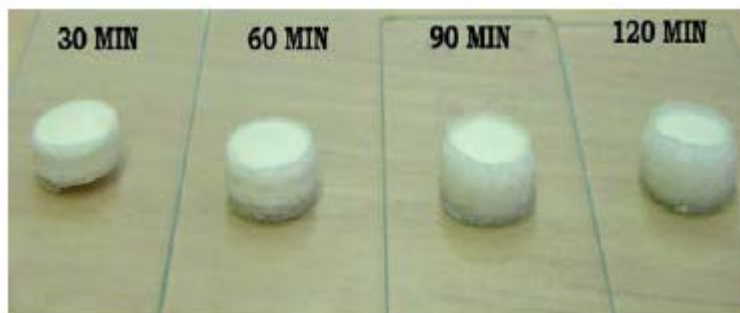
Figure 3. Swelling and Rupture of Surelease Coated Matrices During the Dissolution Run
