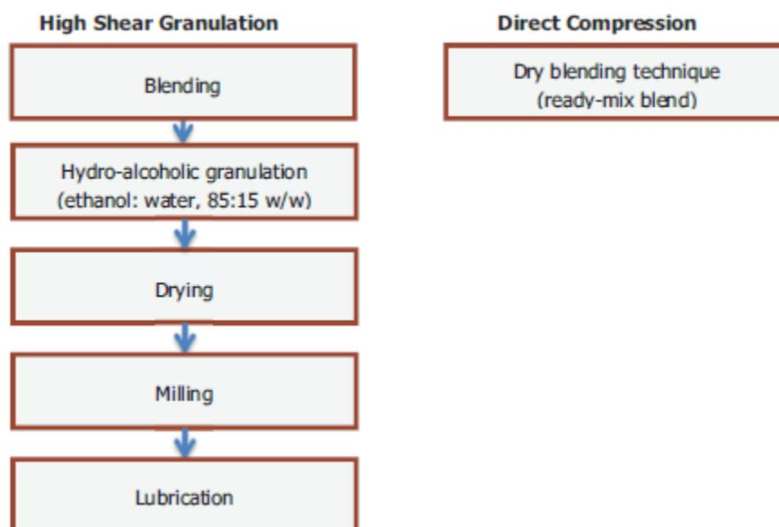
**Figure 2. Manufacturing Process for Push-Pull Osmotic Pump Tablets**
