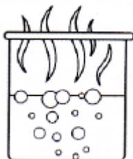
2. Add the METHOCEL™ powder to the heated water with agitation.
