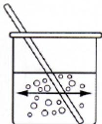
4. For complete solubilization, add the remainder of the water as cold water (or ice) to lower the temperature of the dispersion. Once the dispersion reaches the temperature at which that particular METHOCEL™ product becomes water soluble, the powder begins to hydrate and viscosity increases.
