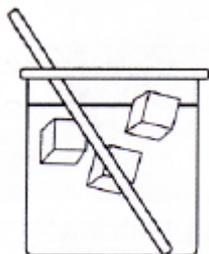
5. Continue agitation for at least 30 minutes after the correct temperature is reached. The solution of METHOCEL™ cellulose ether is now ready to use.
