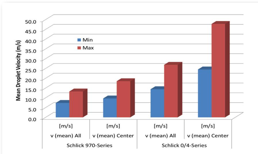
Analysis of data indicated that both the individual and interactive effects of spray rate and atomization air pressure accounted for greater than 60% of the effects on mean droplet size. As expected, an increase in spray rate resulted in an increase in mean droplet size, while increasing atomization air pressure resulted in a decrease in droplet size. These effects were more predominant at moderate to high spray rates, particularly for the production scale nozzle as shown in Figure 5.
