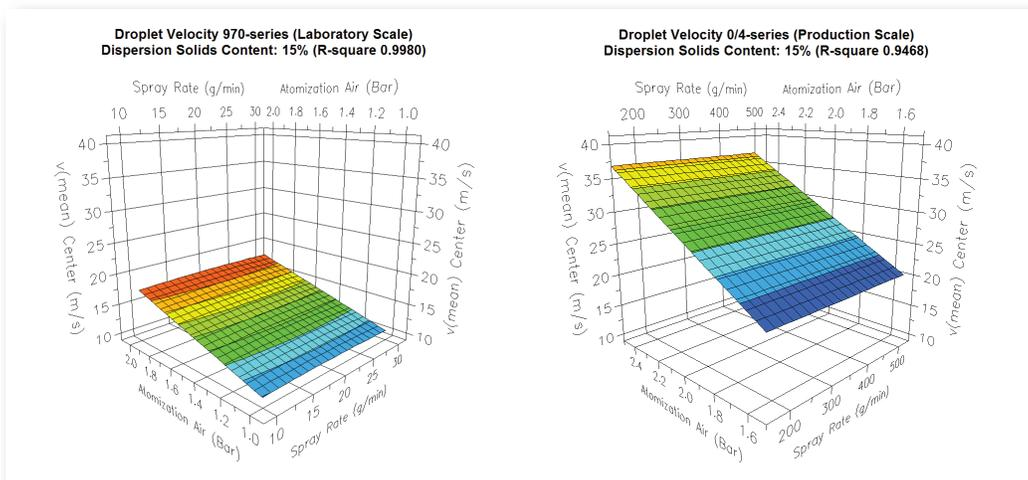
Increases in atomization air pressure, from 1.0 to 2.0 bar at laboratory scale and 1.5 to 2.5 bar at production scale, resulted in an increase in droplet velocity at the center of the spray from 9.7 to 17.4 and 24.5 to 47.8 m/s respectively. As seen in Figure 4, mean droplet velocity for the laboratory and production scale nozzle did not overlap under any test conditions.
