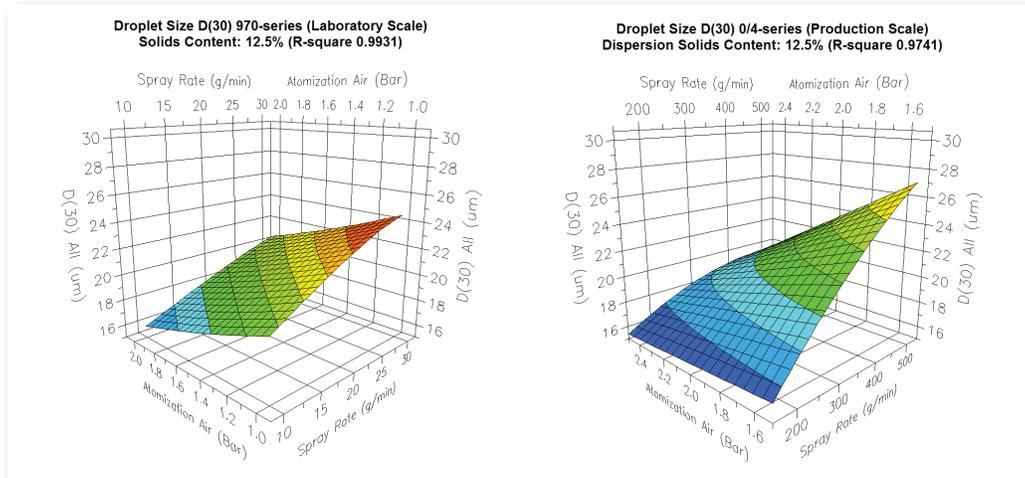
Overlay plots of axial droplet velocity and volumetric droplet diameter, Figure 6, highlights achievable spray characteristics from both laboratory and production scale spray nozzles. Similar droplet velocity from the nozzles tested is unattainable due to differences in air volume consumption. However, it can be seen that similar droplet size can be achieved across broad spray widths.
