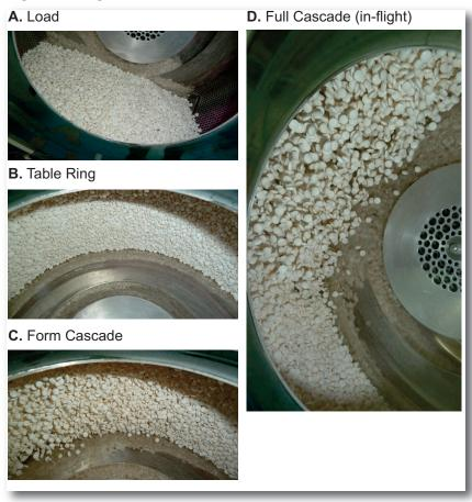
A conventional spray nozzle is directed upwards into the cascade of "in-flight" tablets where essentially their full surface area is available to receive the coating on each pass. A high spray rate relative to the tablet charge is matched by high specific airflows. Filling and discharge is automated and rapid.
