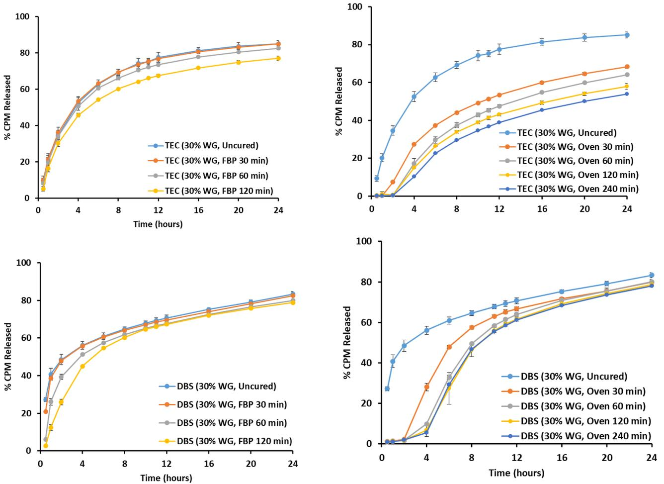
**Figure 3: Effect of Type of Plasticizers and Pore-Formers on CPM Release from BM Coated Beads using Aquacoat® ECD**
