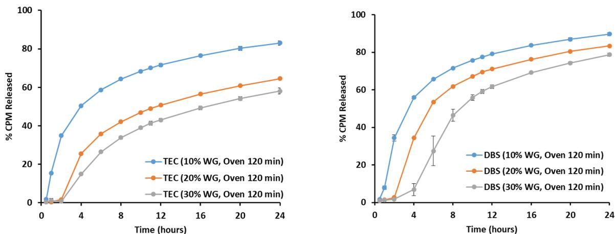
**Figure 2: Effect of Curing on CPM Release from BM Coated Beads using Aquacoat® ECD**
