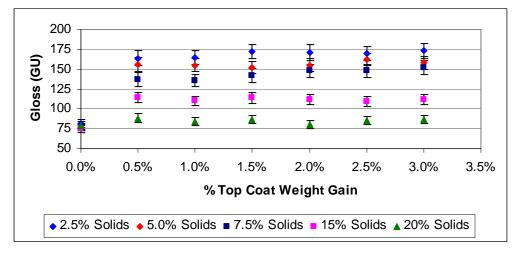
Analysis of the coating time versus gloss showed that higher gloss could be achieved in less time for coatings applied at lower solids. A coating applied at 5% solids achieved a gloss of 156 GU in 20 minutes, whereas, the maximum gloss achieved for all coatings applied at higher solids was 152 GU for a 3% WG applied at 7.5% solids in 80 minutes. A clear coating applied at 2.5% solids achieved a gloss of 164 GU in 40 minutes (Figure 2).
