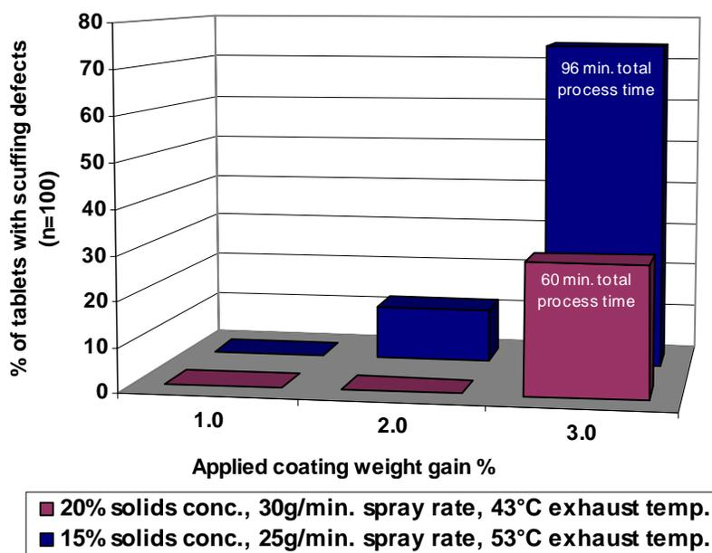
The data also show that the coating process time may be an important factor in the development of scuffing defects. Data from both the laboratory scuffing measurement method and actual coating trials indicate that the longer the tablets rotate in the pan, the greater the development of scuffing defects.
