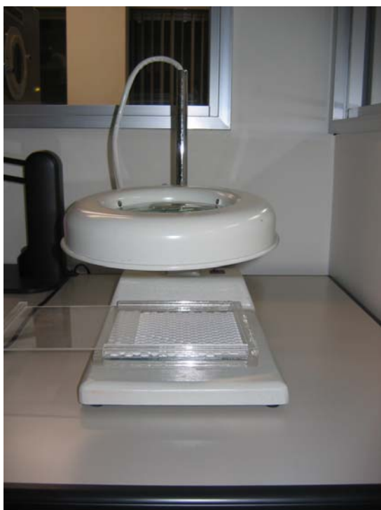
Figure 3. Apparatus for Inspection of Tablet Samples
