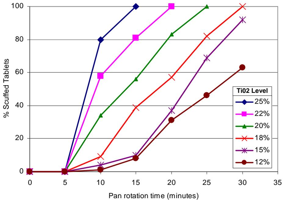
In this test environment, the tablets were simply tumbled and no actual spray was applied to the pre-coated tablets (as opposed to an actual coating environment). These test conditions resulted in much higher levels of scuffing than were observed in subsequent coating trials. The test did, however, demonstrate that adjustments in the level of TiO<sub>2</sub> in the coating formulation can significantly reduce scuffing tendencies.
