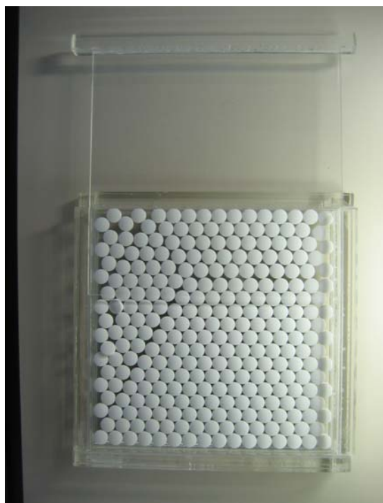
Figure 4. Device for Presenting Tablet Samples for Inspection
