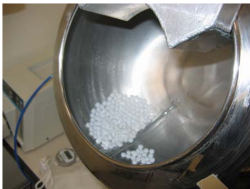
Figure 1. Photos of Tablets Tumbling in the Conventional Stainless Steel Pan
