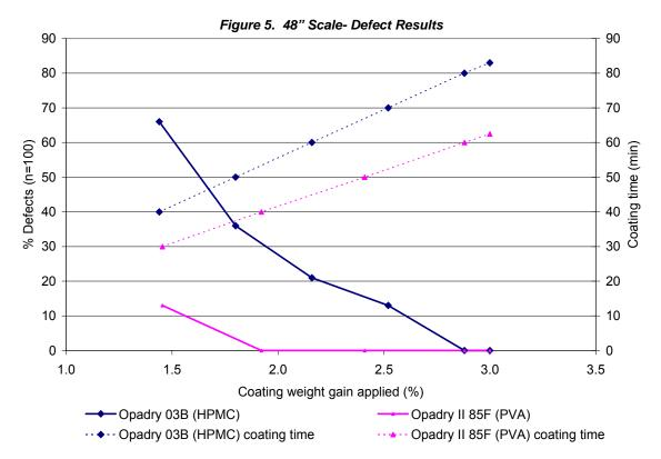
The defect rates for both the HPMC- and PVA-based coating systems were significantly lower on production scale than seen on laboratory scale. This is consistent with the findings of Mueller et al. who investigated the influence of scale-up on the abrasion of tablets and postulated that larger pan loads resulted in less tablet impacts with the pan walls and baffles.<sup>4</sup>
