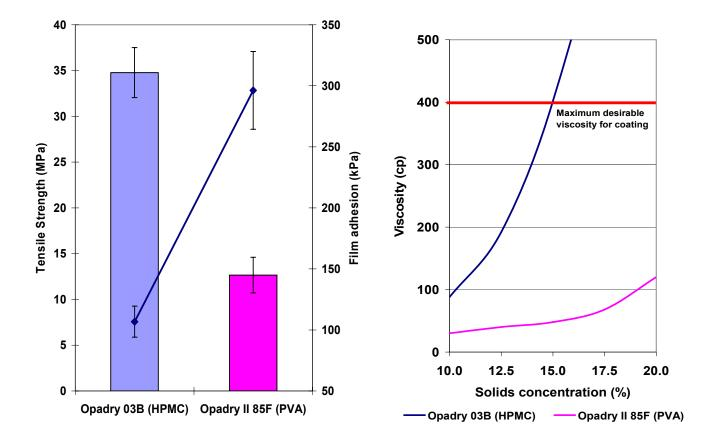
Historically, film strength has been shown to be a critical attribute in reducing the incidence of coated tablet edge defects.<sup>1</sup> It is also recognized that film adhesion plays an equally important role and a robust coating formulation must balance each of these factors.<sup>2</sup>
