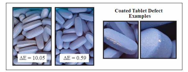
The laboratory-scale coating trials were conducted in 24" full-perforated pan (O'Hara Technologies Labcoat II). Production-scale trials were conducted in a 48" fully-perforated pan (O'Hara Technologies Fastcoat). Both pans were fitted with 1.0 mm spraying systems VAU anti-bearding spray guns. The target coating weight gain for all trials was 3.0%.
