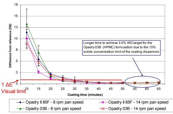
Color development data exhibited similar trends across the four laboratory scale trials. At early stages in the trials (10-15 min), higher pan speeds were seen to improve color uniformity. Both the HPMC-based and PVA-based coating systems achieved target color and uniformity in ~40 minutes. The HPMC-based took 15 minutes longer to reach the target 3.0% weight gain due to the reduced solids concentration of the coating suspension.
