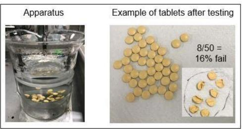
Samples were also tested for dissolution according to USP Aspirin Delayed Release Tablets monograph.
