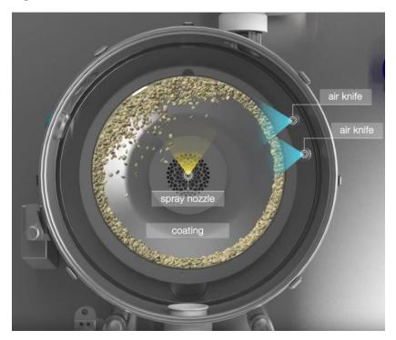
In traditional coating pans, it has been demonstrated that the coating is always thicker on the face as compared to the edge or end of the tablet since they are closely packed and not able to freely rotate as they pass through the spray zone.<sup>1</sup>
