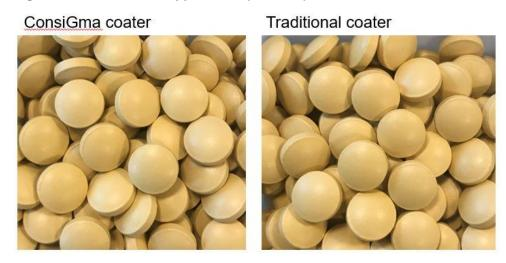
The ConsiGma coated tablets passed acid resistance testing at 8% WG compared to the traditionally coated tablets that passed at 10% WG (Figure 4).
