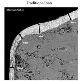
**Table 1: Coating Thickness Measurements**
