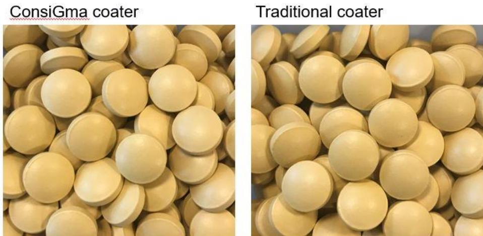
The ConsiGma coated tablets passed acid resistance testing at 8% WG compared to the traditionally coated tablets that passed at 10% WG (Figure 4).
