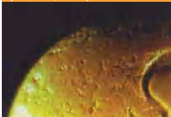
Figure 7 Surface of a film coated tablet containing a high level of a superdisintegrant.
