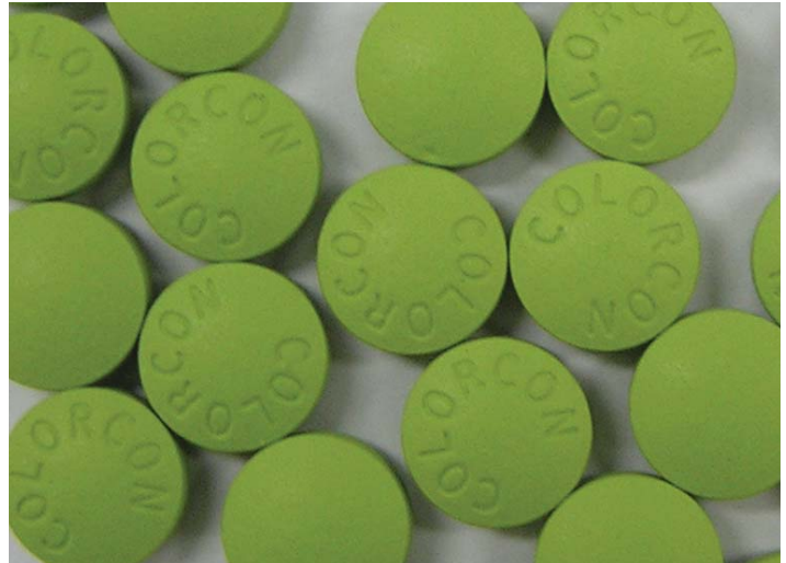
Figure 5 - Picture of XCH Film-Coated Tablets Formula 2 (4% Starch 1500) & Coated with Opadry II 85G 61282 Green
