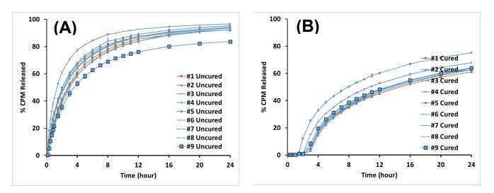
Figure 2. Dissolution Data for All Runs Uncured (A) and Cured (B)
