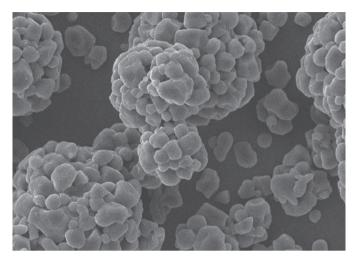
SEM image of StarCap particles
