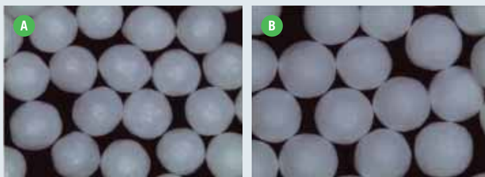
Figure 3: A: Lansoprazole drug-layered sugar spheres; B: Sugar spheres with 40% WG Acryl-EZE II enteric coating
