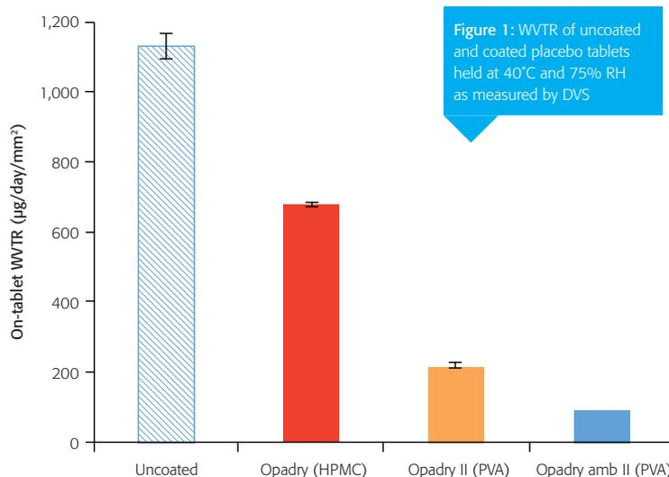
Figure 1: WVTR of uncoated and coated placebo tablets held at 40°C and 75% RH as measured by DVS
