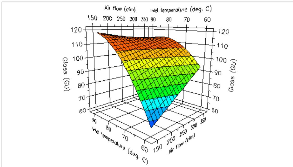
**Figure 3. Effect of Inlet Temperature and Airflow on Gloss at 25% Solids Concentration**
