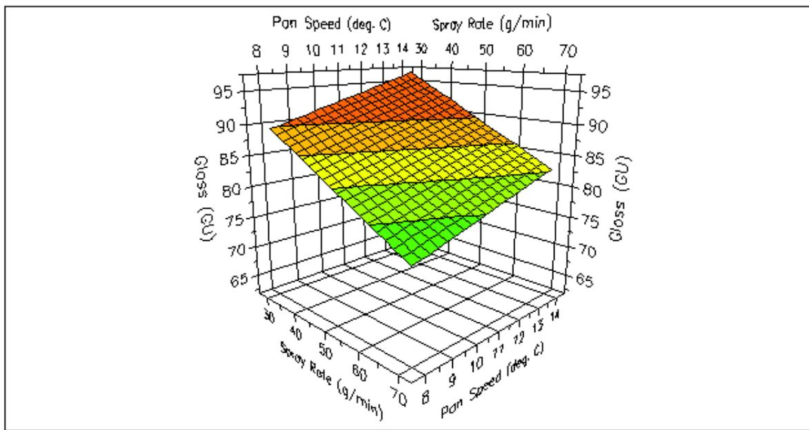
**Figure 7. Effect of Pan Speed and Spray Rate on Gloss at 30% Solids Concentration**
