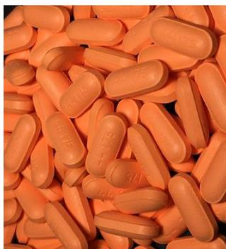
Placebo caplets were coated in the O'Hara Fastcoat 48" pan using the processing conditions described in Table 2. The production scale coating trial produced tablets with excellent appearance as shown in Figure 5. A comparison of the tablet gloss and surface roughness, shown in Figures 6 and 7, indicates that comparable performance can be achieved on both the 24" and 48" scale.
