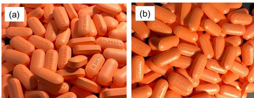
**Figure 6: Gloss Coated of Placebo Caplets Coated with Pigmented Opadry EZ and Opadry EZ Clear on the 24" and 48" Scale**
