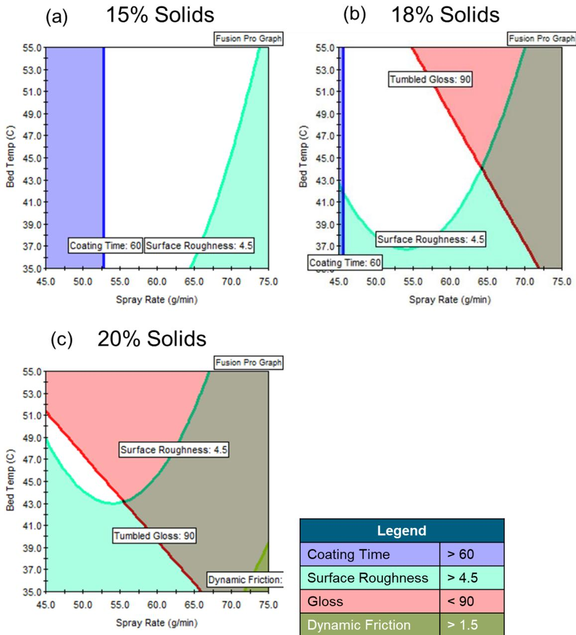
Confirmation runs were performed on APAP caplets in the 24" scale to confirm the DoE model. The spray rate and bed temperatures were chosen to provide ideal coating performance at 15, 18 and 20% solids as shown in Table 3.
