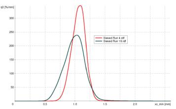
These runs also produced the tightest distribution of bead sizes and the widest distribution of sizes, reported as the span by the Camsizer respectively. Figure 4 shows these distributions. Run 19 produced a wider distribution because the bead shape impacted the sieving process. The deviation from sphericity made the sieving process more difficult, resulting in a wider distribution.
