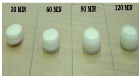
Figure 3. Swelling and Rupture of Surelease Coated Matrices During the Dissolution Run
