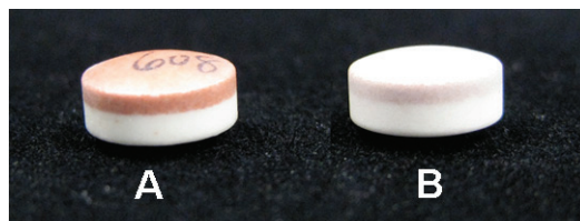
Figure 4. Example of Clear Acceptable (A, Trial 9) vs. Opaque Unacceptable (B, from a separate study) SPM Opacity
