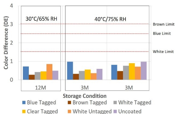
Figure 2. Color Difference (DE) for Tagged and Untagged APAP Tablets Over Stability Through 12 Months 30°C/65% RH or 6 Months 40°C/75% RH
