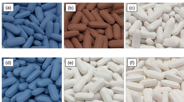
Figure 2. Color Difference (DE) for Tagged and Untagged APAP Tablets Over Stability Through 12 Months 30°C/65% RH or 6 Months 40°C/75% RH
