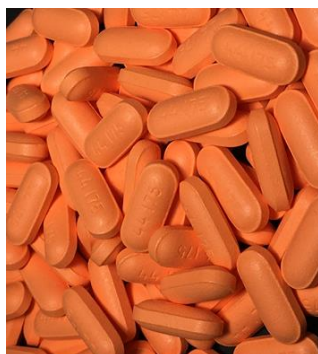
Figure 4: APAP Caplets Coated in the 24" Pan with Pigmented Opadry EZ at 18% Solids
