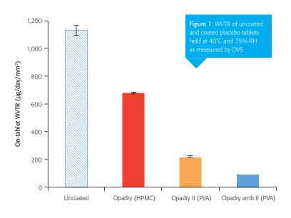
DVS monitors weight variation due to moisture uptake in an environment of changing humidity and temperature. It has previously been shown that lower uptake values can lead to better moisture barriers (3).
