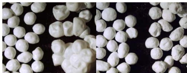
Figure 4: Optical Microscope Images of Pellets before (MPs on the Left) and After Exposure to pH 4.5 (MPs on the Right): (A) without Fumed Silica; (B) with 1.0% Fumed Silica Sprayed.
