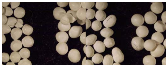
Figure 3: Optical Microscope Images of Pellets Before (MPs on the Left) and After Exposure to pH 1.2 (MPs on the Right): (A) without Fumed Silica; (B) with 1.0% Fumed Silica Sprayed
