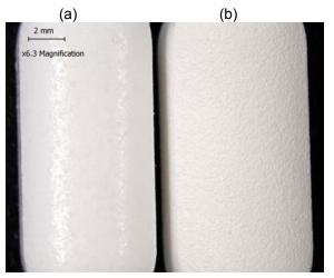
Figure 4. Appearance of (a) Uncoated and (b) Opadry II Coated Metformin HCI PEO Matrix (X6.3)
