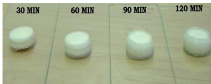
Figure 3. Swelling and Rupture of Surelease Coated Matrices During the Dissolution Run
