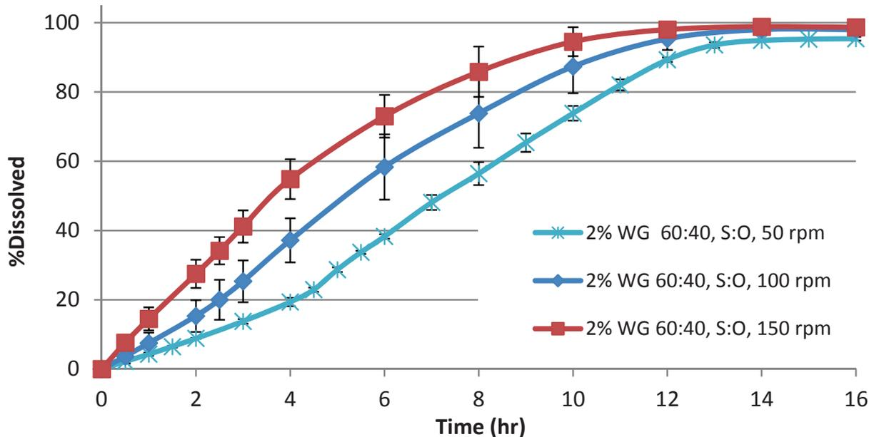
Figure 3. Dissolution Profile of HCTZ 200 mg ER Tablets Coated with BM Coating Consisting of Surelease® and Opadry® at 60:40 Ratio and 4% WG.
