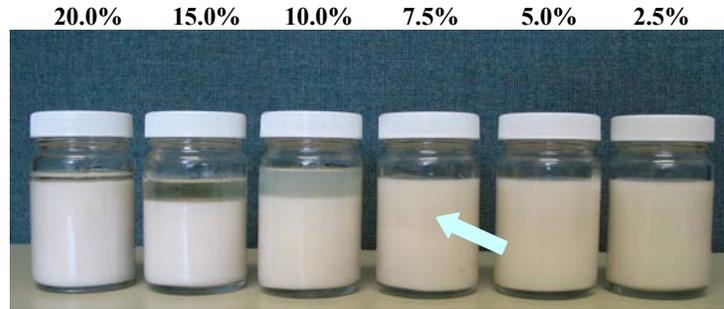
**Figure 2. Effect of HPMC Concentration (2.5 – 20% w/w) on (a) Sedimentation and (b) Viscosity Curves**
