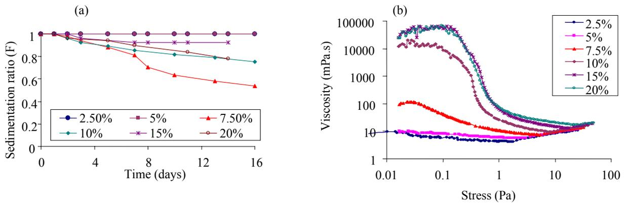
EC dispersions containing 10% w/w or more HPMC exhibited pronounced shear thinning; the rheological profiles are representative of a system with network formation. The zeta potential of freshly prepared EC-HPMC dispersions, with the exception dispersion containing 20 %w/w HPMC, were similar to dispersion without pore-former (Figure 2). After 4 weeks of storage, dispersions which showed sedimentation were redispersed before aliquot volumes of sample were diluted for zeta potential measurement.
