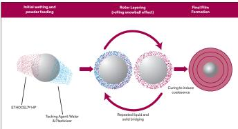
Figure 5. The dry powder layer process.
