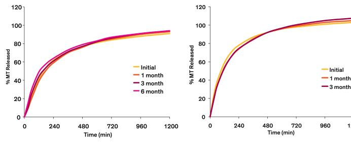
Figure 15. Drug release stability of ETHOCEL HP coated Metoprolol tartrate multipaticulates prepared with 40% DBS plasticizer and dynamically cured at 40°C product temperature.
