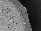
Figure 6. Cross sectional image (left) and magnified view (right) of ETHOCEL™ HP barrier membrane formed from dry powder rotary coating process.
