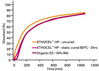
Figure 10. Metoprolol tartrate drug release for ETHOCEL™ HP rotary coatings and organic ETHOCEL™ spray coatings
