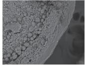
Figure 4. Cross sectional image (left) and magnified view (right) of ETHOCEL™ barrier membrane formed from solvent solution.
