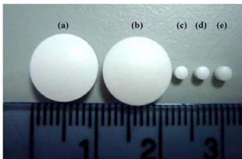
The mechanical strengths of the mini-tabs improved significantly after the application of a seal-coat. Breaking force increased from 1.1 kp (uncoated) to 3.3 kp (seal-coated) and friability was reduced from 0.24% to less than 0.01% respectively.
