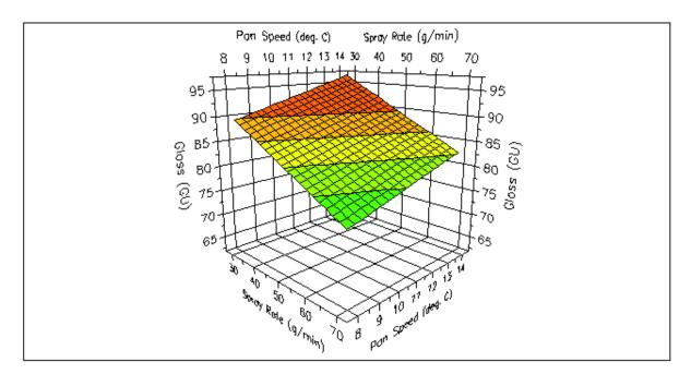
Figure 6. Effect of Pan Speed and Spray Rate on Gloss at 15% Solids Concentration
