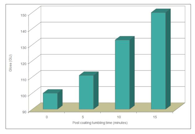
Further increases in gloss were not observed at tumbling times > 15 minutes. The increase in gloss with postprocess tumbling may be attributed to the physical properties of the film coating composition used in this study, which has been previously shown to have a higher degree of "slip" than other coating systems. This higher slippage during tumble in the pan allows further smoothing of the coating surface after the spray has been stopped.
