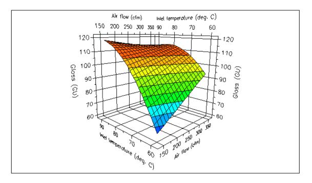
Figure 2. Effect of Inlet Temperature and Airflow on Gloss at 15% Solids Concentration
