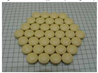
Figure 3. Coated Tablet Appearance (10% Weight Gain)
