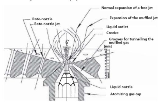
Figure 2. Schematic of Spray Nozzle and Air Distribution Plate
