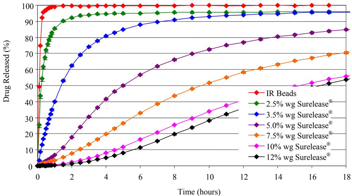
**Figure 4. Dipyridamole Dissolution from Pellets Coated with Surelease<sup>®</sup> Containing PVA or PVA/PEG**
