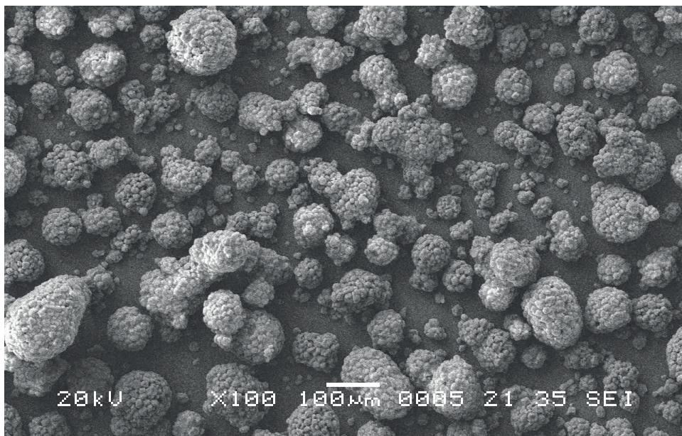
SEM image of StarTab particles
