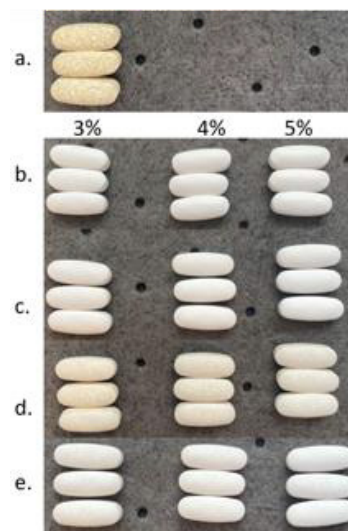
Figure 1. (a) Uncoated Multivitamin, (b) Multivitamin Tablets coated with Nutrafinish TiO 2 , (c) Nutrafinish High Opacity, (d) Experimental, and (e) Nutrafinish Label Friendly
