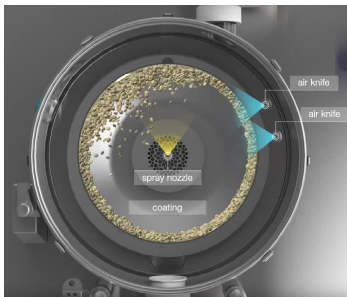
Figure 1: Tablet Motion in the ConsiGma Coater
