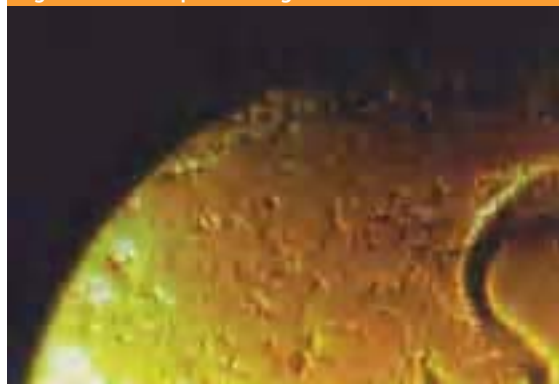
Figure 7 Surface of a film coated tablet containing a high level of a superdisintegrant.
