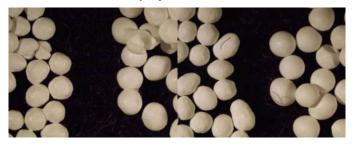
Figure 4: Optical Microscope Images of Pellets before (MPs on the Left) and After Exposure to pH 4.5 (MPs on the Right): (A) without Fumed Silica; (B) with 1.0% Fumed Silica Sprayed.
