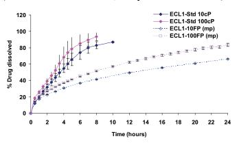
Figure 4. Dissolution Profiles of Theophylline Tablets (ECM1)(TP/EC/MCC = 1:1:1, Compression Force: 10kN)
