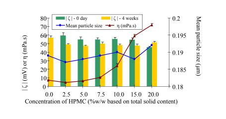
Figure 3. Effect of HPMC Concentration on Zeta Potential ( $|\zeta|$ ), Particle Size, and Viscosity ( $\eta$ ) of EC Dispersion
