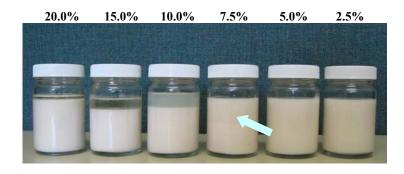
Figure 1. Surelease Dispersions Containing 2.5 – 20% w/w HPMC
