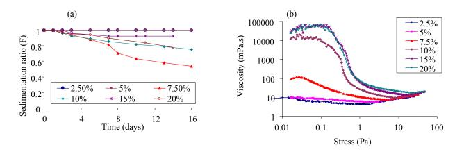
EC dispersions containing 10% w/w or more HPMC exhibited pronounced shear thinning; the rheological profiles are representative of a system with network formation. The zeta potential of freshly prepared EC-HPMC dispersions, with the exception dispersion containing 20 %w/w HPMC, were similar to dispersion without pore-former (Figure 2). After 4 weeks of storage, dispersions which showed sedimentation were redispersed before aliquot volumes of sample were diluted for zeta potential measurement.
