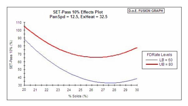
Figure 3. SET Performance vs, Solids and Fluid Delivery Rate
