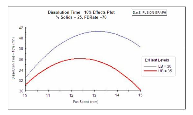
Figure 7. Dissolution Time vs. Pan Speed and Exhaust Heat
