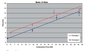
Figure 3: Tablet dissolution
