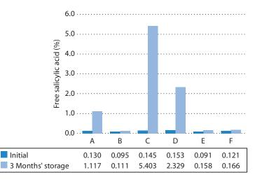
After 3 months of storage ... some of the tablets containing CCS or SSG exhibited softening of the film coating and sticking of the tablets to one another within the HDPE bottles.
